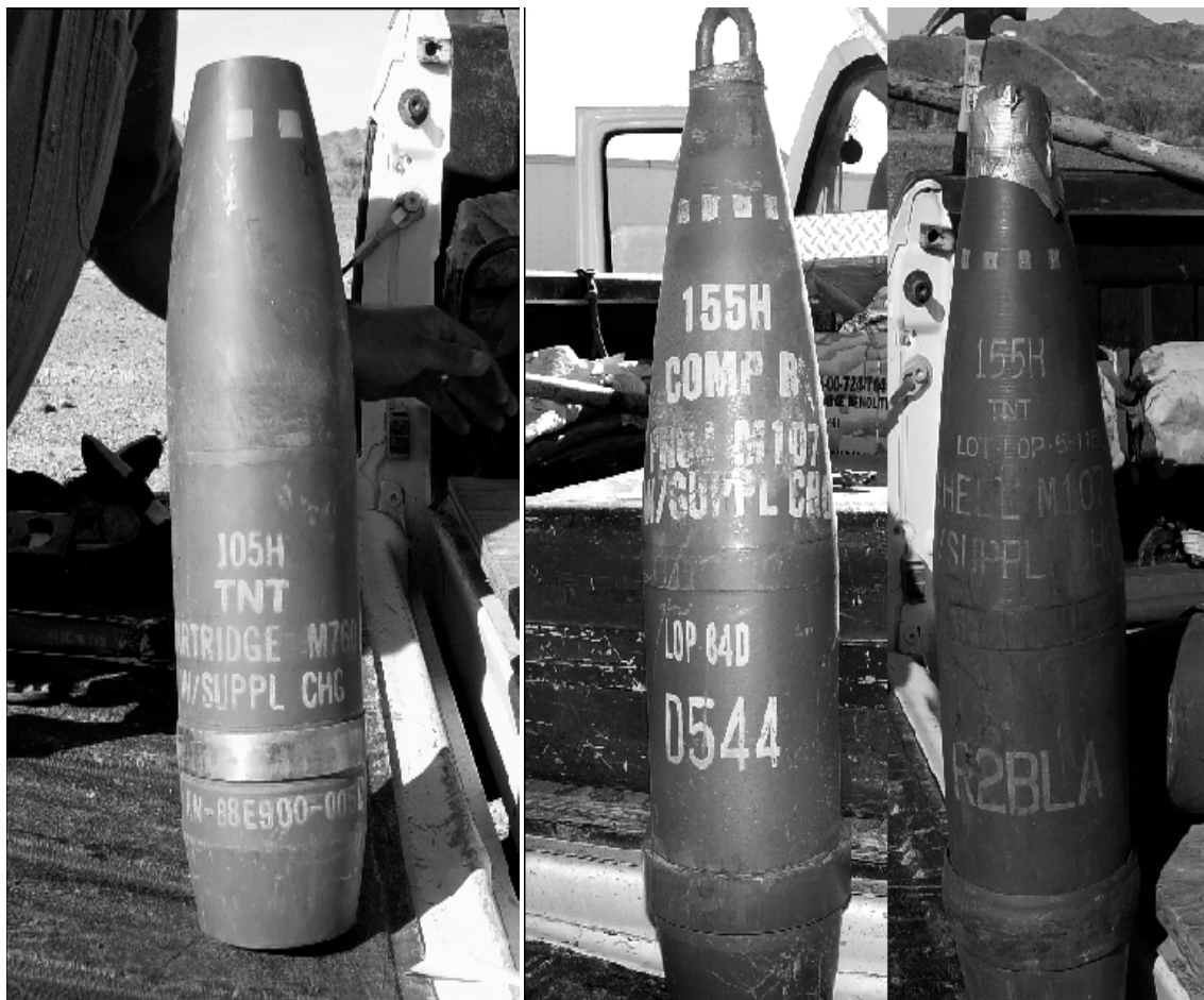
Figure 3. M760 105 mm Cartridge (left), M107 155 mm Comp-B (center), and TNT Cartridge (left).
