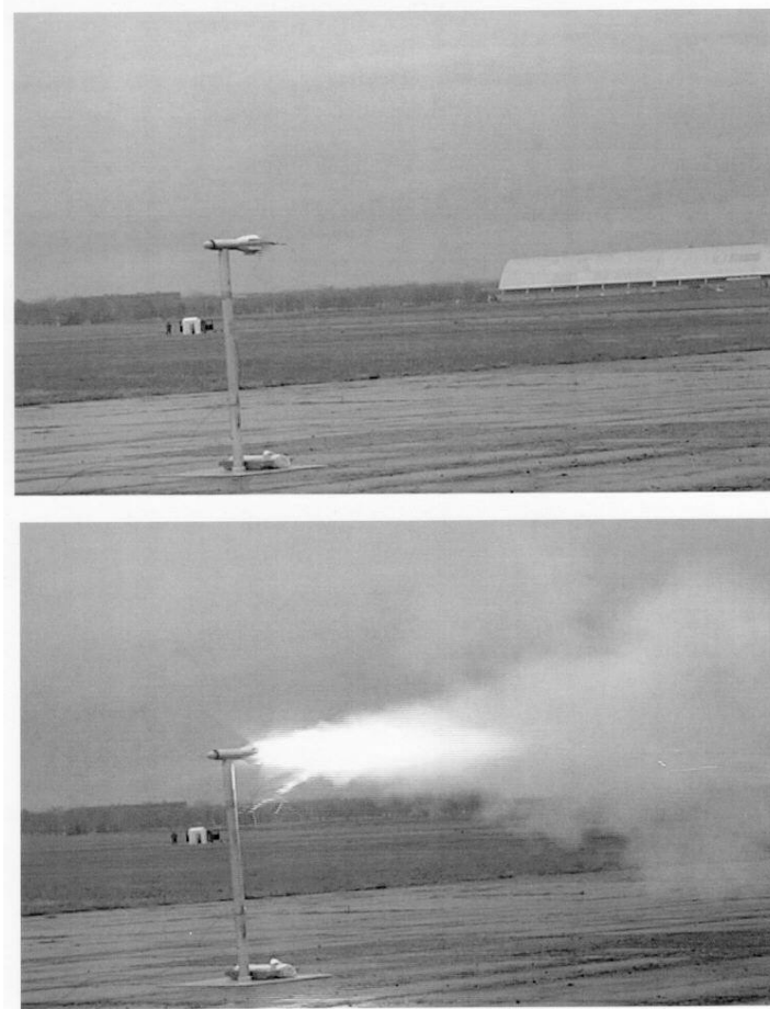
Figure 6. Test stand with rocket un-ignited (top) and ignited (bottom)
