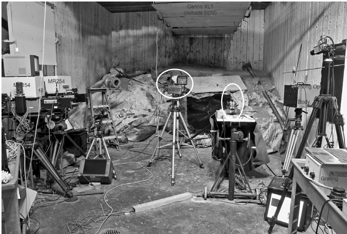
Figure 7. The instrument arrangement for TPL muzzle flash tests. The Phantom camera is at the approximate center of the image (left ellipse). The test pistol is slightly below and to the right (right ellipse).
